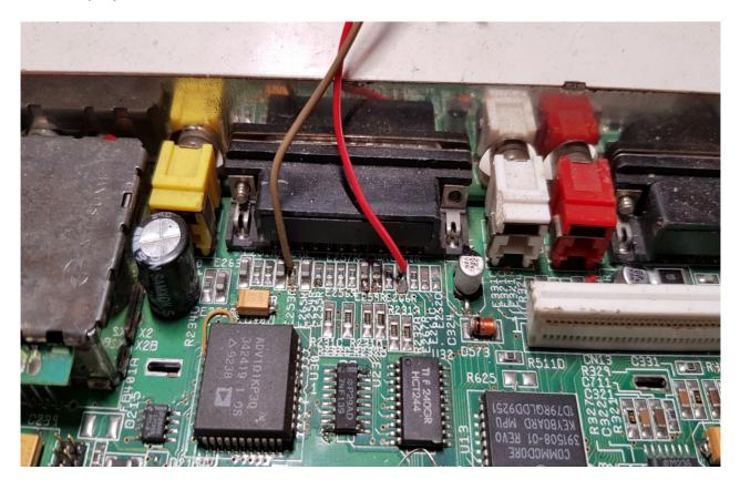
Solder bootselector wires to A1200 board:
